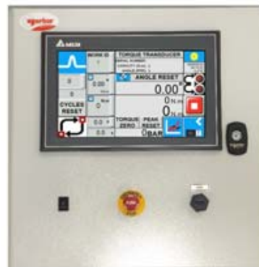
Tool controller Q4673 with 10" HMI & remote pendant 61142.1000
