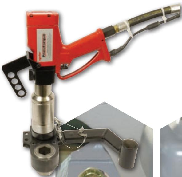
In this typical engineer to order application, the train operator was struggling to tighten the bolts pocketed into this casting. Norbar's solution was this special offset gearbox.
