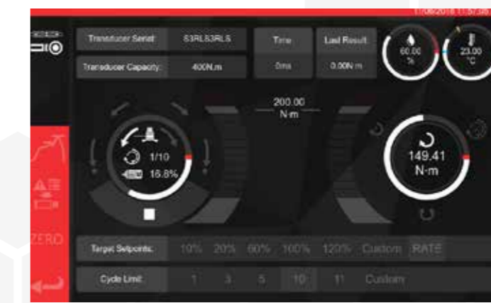
Tool cycling and adjustment whilst in operation
