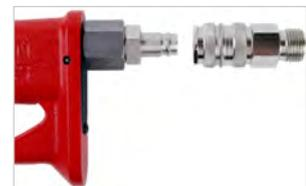
Connect the inlet side of the lubro control unit (Figure 1-B) to the air supply (Figure 1-C) using a minimum hose size of 1/2" bore (12mm). Avoid using 1/2" bore hoses of longer than 5 meters from the supply to the pressure regulator unit as this will reduce the performance of the tool.
