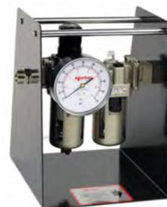
**IMPORTANT:** THE WRENCH MUST BE FREE RUNNING WHILE ADJUSTING THE AIR PRESSURE TO GIVE THE CORRECT SETTING.
