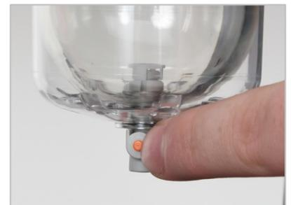
**FIGURE 5 – Draining Condensate**
