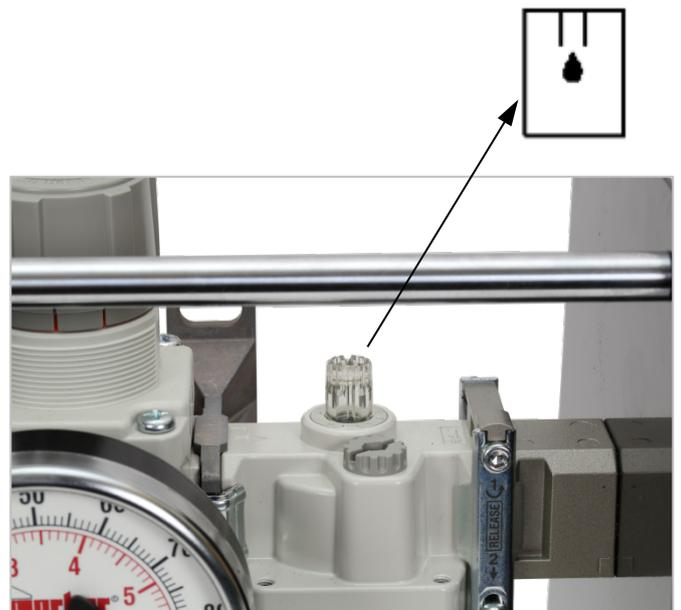
**FIGURE 3 – Lubricator Flow**
