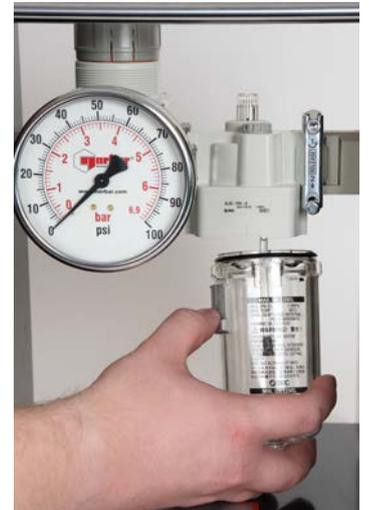
**FIGURE 4 – Lubricator Bowl Replacement**
