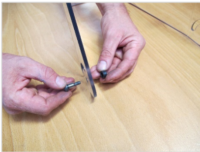
FIGURE 6 – Pairing the Neoprene Washers with Shoulder Bolts
