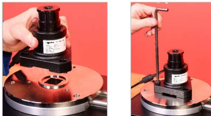
FIGURE 14 – Fitting an FMT Transducer
