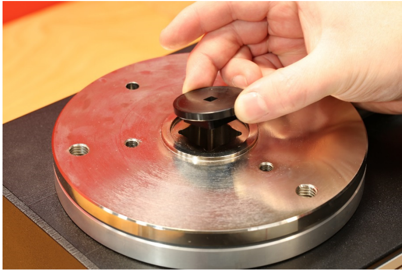
FIGURE 26 – Inserting Square Adaptor
