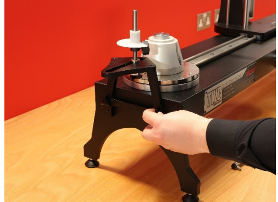
FIGURE 28 – Attaching Short Length Reaction Plate
