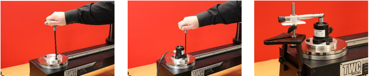
FIGURE 30 – Attaching FMT 2 to FMT 25 Adaptor Kit
