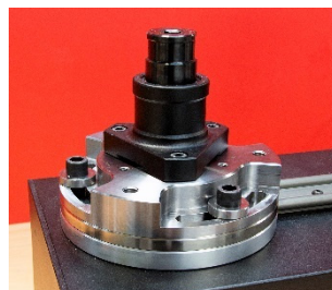
FIGURE 32 – Attaching TWC Angle Offset Plate
