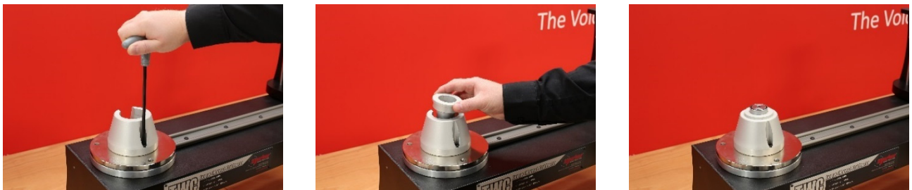
FIGURE 27 – Fitting Static Transducer Support Kit
