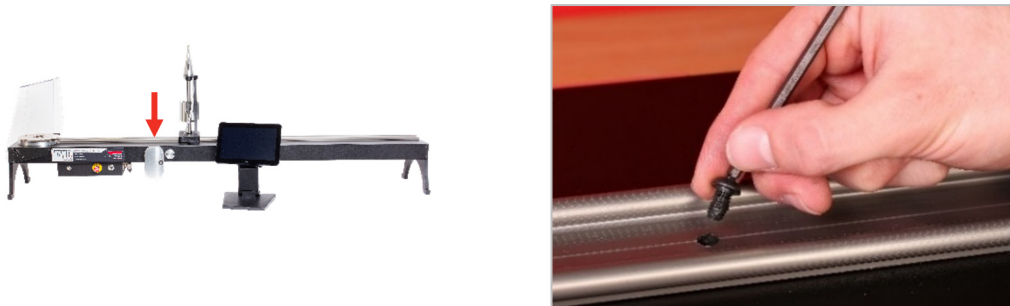
FIGURE 21 – Removing Button Head Cap Screw
