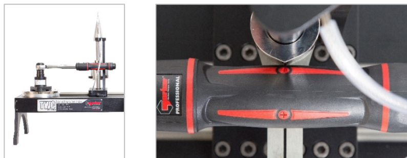
FIGURE 16 – Locating a Torque Wrench
