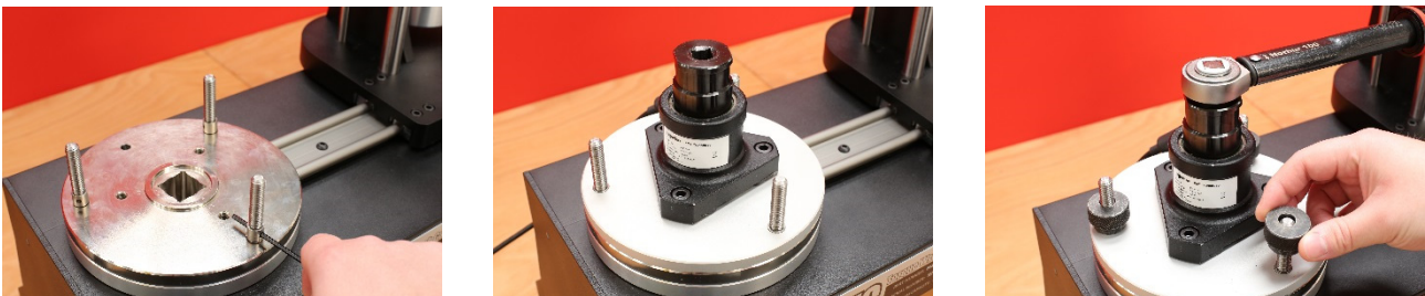
FIGURE 31 – Attaching FMT Quick Release Kit
