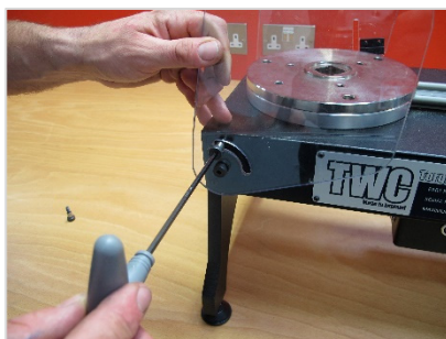
FIGURE 7 – Fitting the Guard
