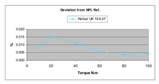
Figure 3. deviation of a 100 N·m transducer from the NPL reference value.
