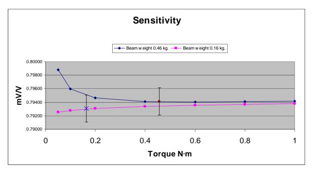
Figure 2. Sensitivity of a 1 N·m transducer calibrated with unsupported calibration beams.
