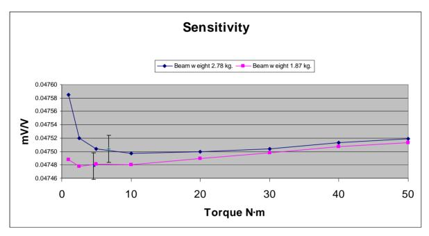
Figure 1. Sensitivity of a 50 N·m transducer calibrated with unsupported calibration beams.
